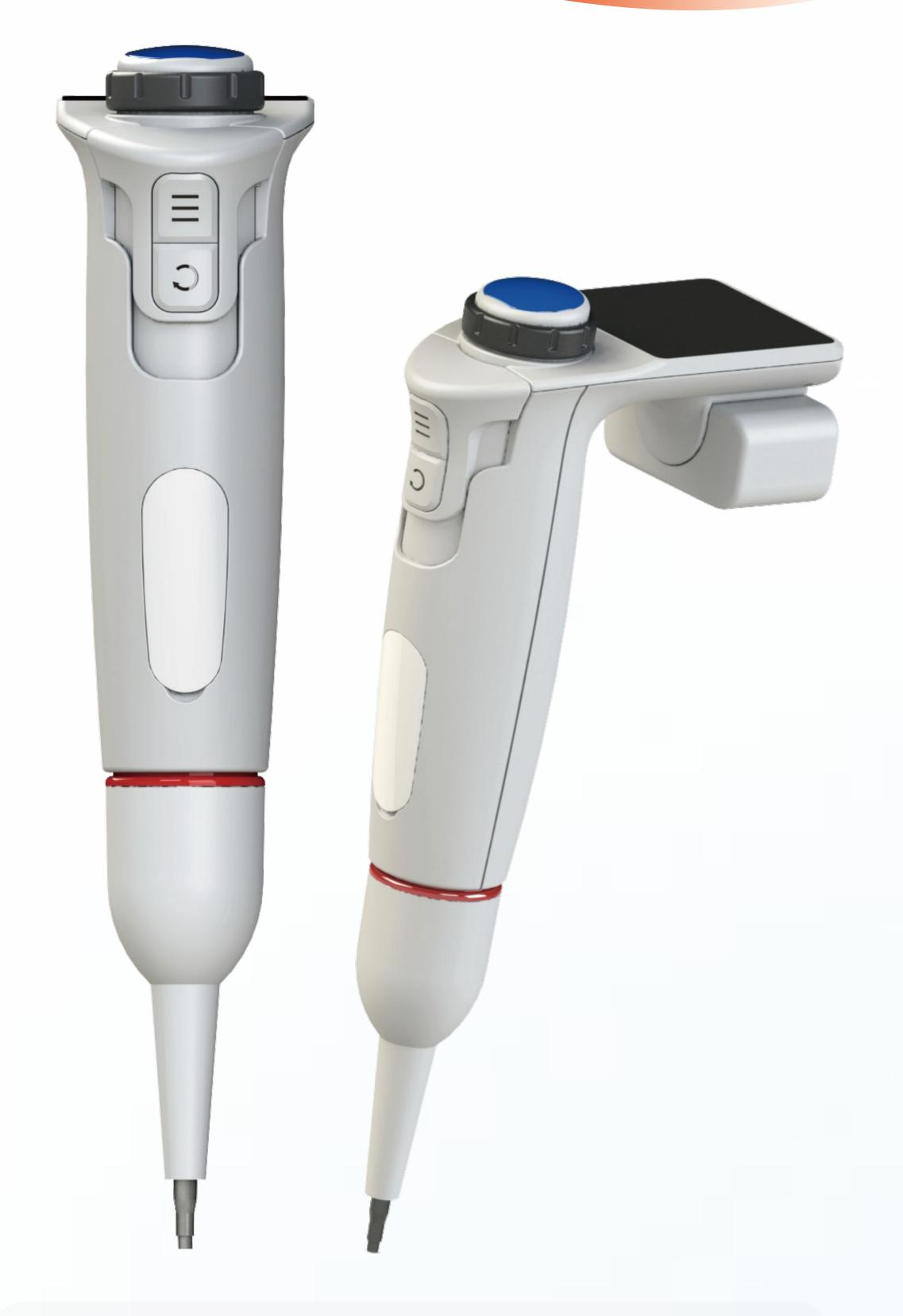
The onepipet® electronic pipette is an electronic volumetric instrument designed to measure and transfer liquids precisely and safely. It can measure and transfer volume from 0.1 ul to 5000 ul depending on the model.
