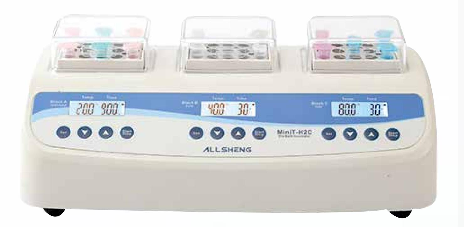
The Tri-Block Dry Bath is ideal for incubation of samples at three different temperatures, in a single compact item. The three chambers are separated by an insulated wall and are controlled separately, allowing Tri-Block to serve as three dry bath incubators in one unit.
