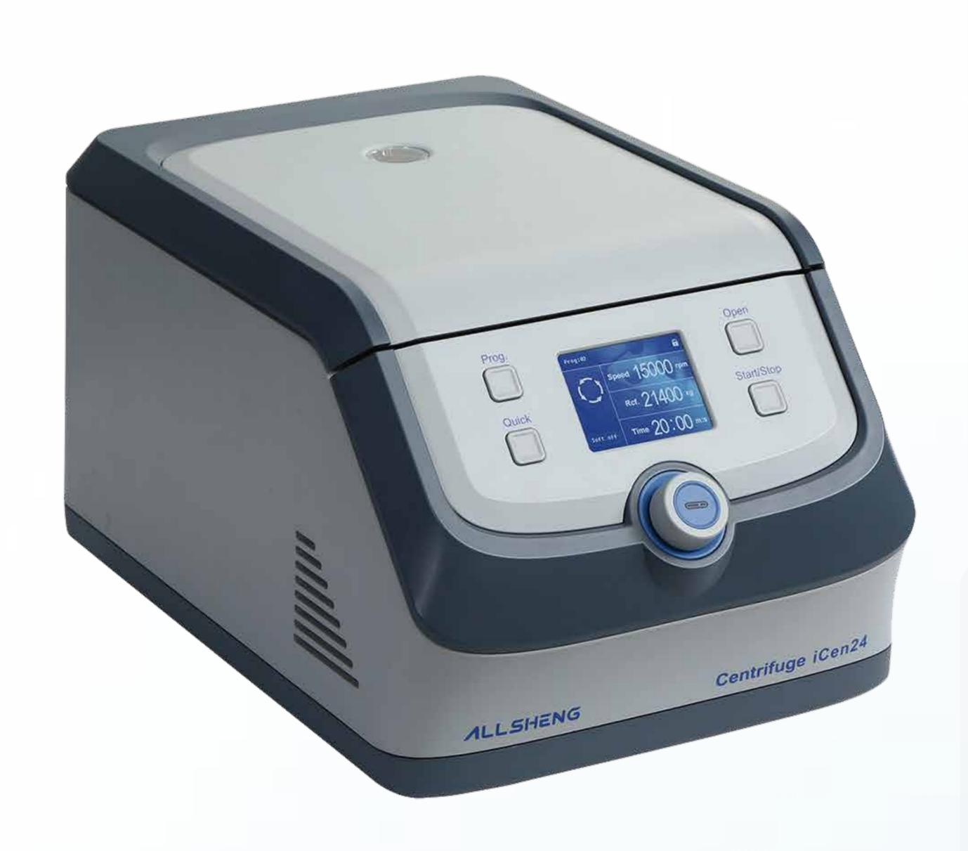
High Speed Centrifuge ICEN-24 is a compact benchtop high speed unit with a 24-tube rotor. The max speed can reach 15000 rpm (21,400×g). It features a separate short spin key for quick centrifugation.
